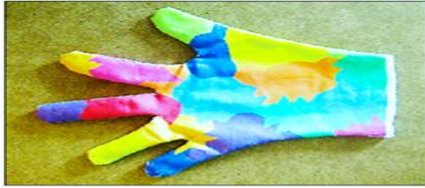
Figure 6. Color-based recognition using a glove marker
