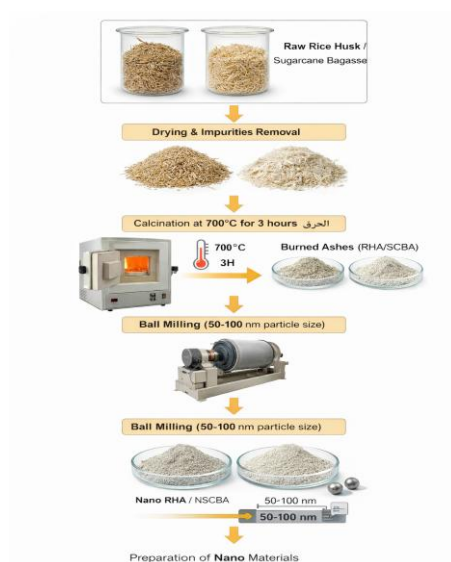
Fig. 2. Preparation of nano ashes
