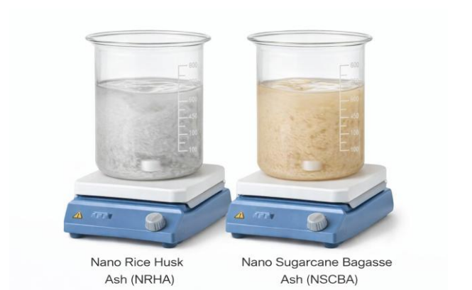
Fig. 3. Dispersion of nano materials using a magnetic stirrer
