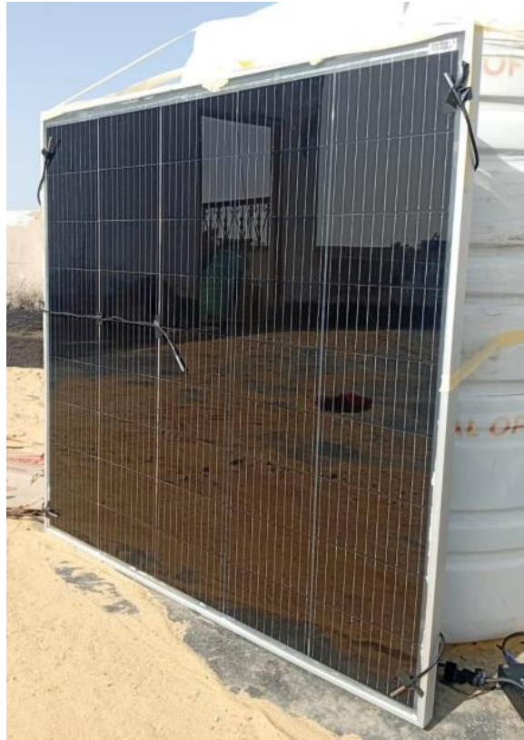
Figure 4. Jet Solar JSM-195SP module used for the localized electrical field test at the Damanhour study site.
