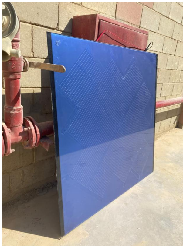
Figure 5. JA Solar JS-190W-Special module used as the second PV option in the comparative field and simulation assessment.
