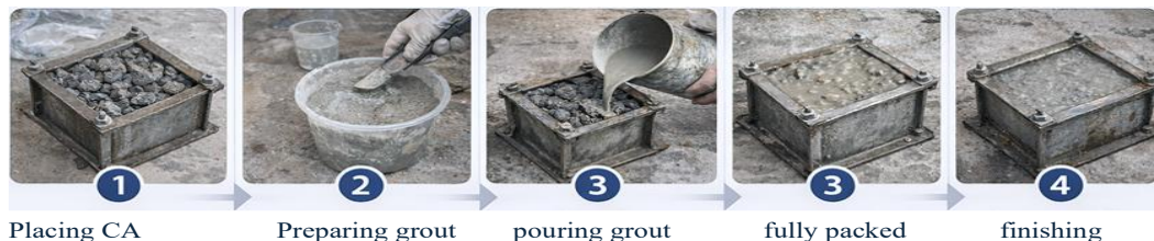
Figure 2. Casting procedures of prepacked HSC
