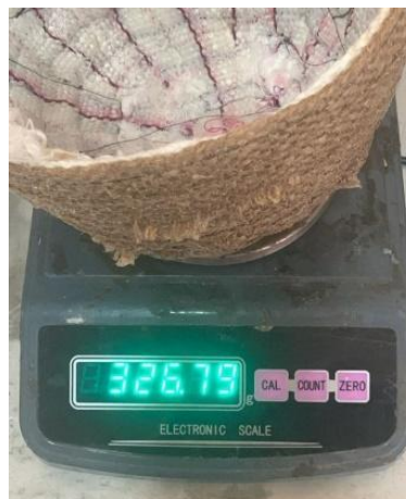
Figure 3: Direct physical mass quantification of the hybrid textile-polymer composite helmet (H2 configuration) utilizing a calibrated laboratory electronic scale.
