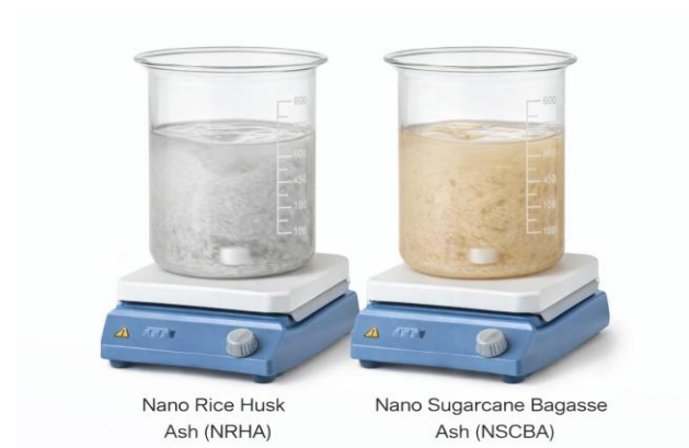
Fig. 3. Dispersion of nano materials using a magnetic stirrer
